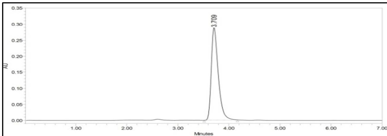
Figure No.3: Typical chromatogram of Metaxalone tablet
