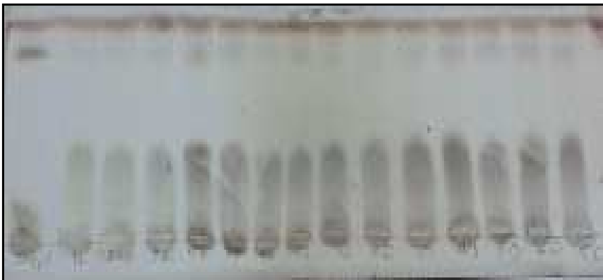
Figure No.5: Photograph of the TLC plate alfalfa seed and the elicited sprouts extracts with different concentrations of MO extract in light and dark, using solvent system (7.5 methylene chloride: 2.5 methanol)
